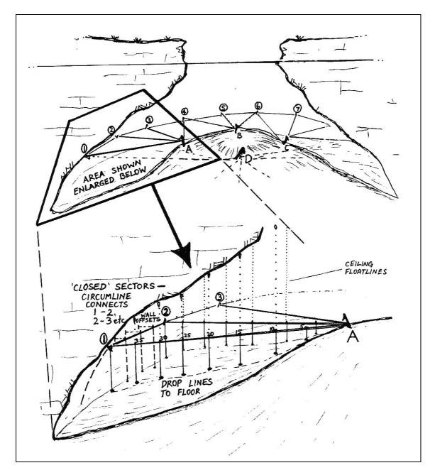
A (closed) **RADIAL SURVEY** involving numerous wall stations and diverging rays at the same level, and offsets from those rays ("Ten-Eighty Sinkhole" Project, SAUSS Inc.)
