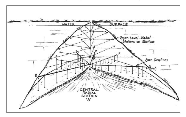
A multi-level (open) **RADIAL SURVEY** from a single (central) reference station; the technique used in mapping "The Shaft" (5L158) by the CDAARG (1983)
