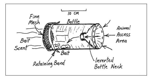
A Basic Inverted-Cone Mesh Trap
