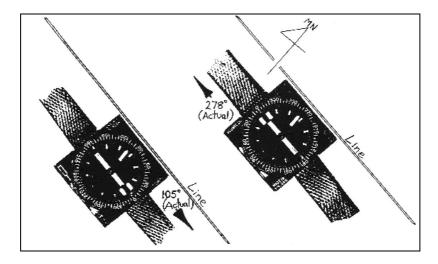
**ACTUAL** bearings as indicated by the North-seeking needle e.g. a standard diver's compass
